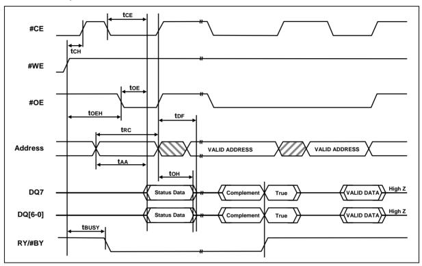
Figure 8-19 Data# Polling Timing Waveform (During Automatic Algorithms)
