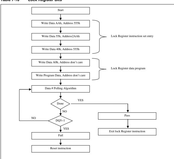
Figure 7-2 Lock Register Program Algorithm
