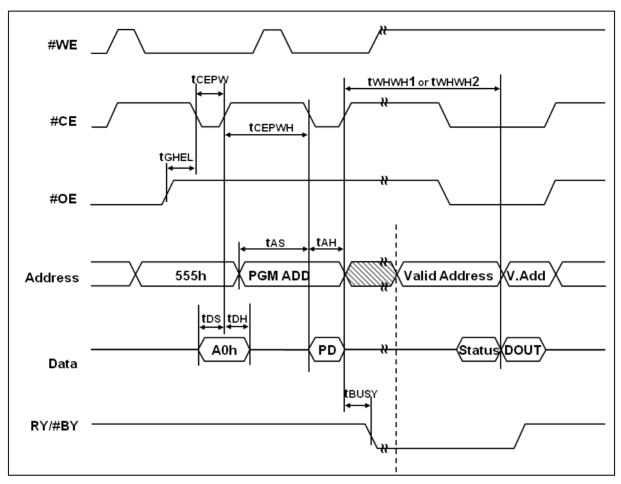
Figure 8-15 #CE Controlled Write Timing Waveform
