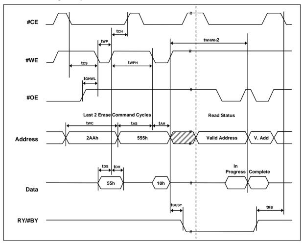
Figure 8-8 Automatic Chip Erase Timing Waveform
