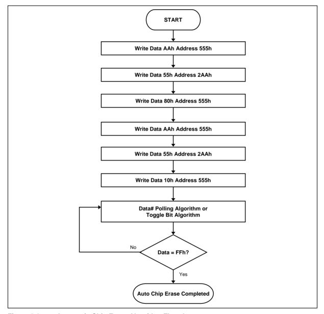
Figure 8-9 Automatic Chip Erase Algorithm Flowchart
