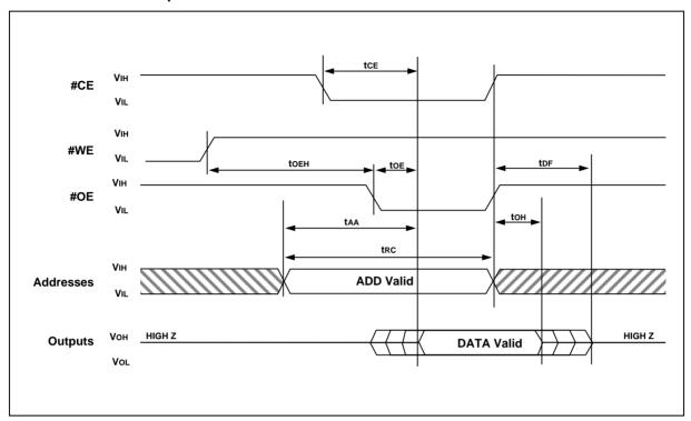
Figure 8-6 Read Timing Waveform
