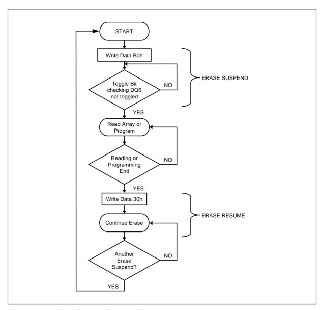
Figure 8-12 Erase Suspend/Resume Flowchart
