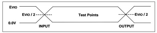
Figure 8-4 Switching Test Waveform
