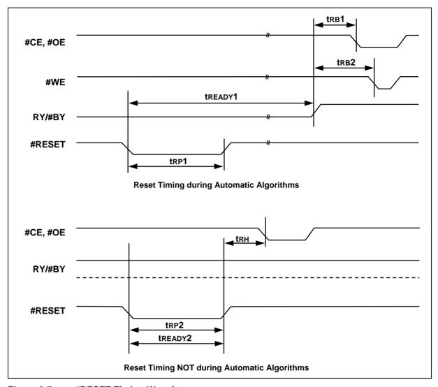
Figure 8-7 #RESET Timing Waveform
