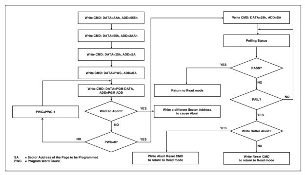
Figure 8-27 Write Buffer Program Flowchart
