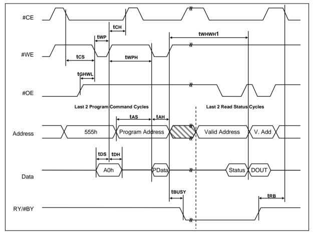
Figure 8-13 Automatic Program Timing Waveform
