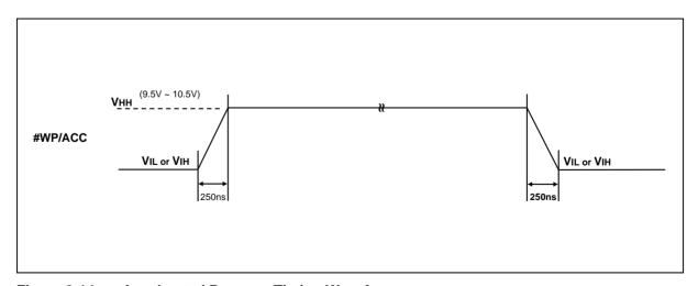
Figure 8-14 Accelerated Program Timing Waveform
