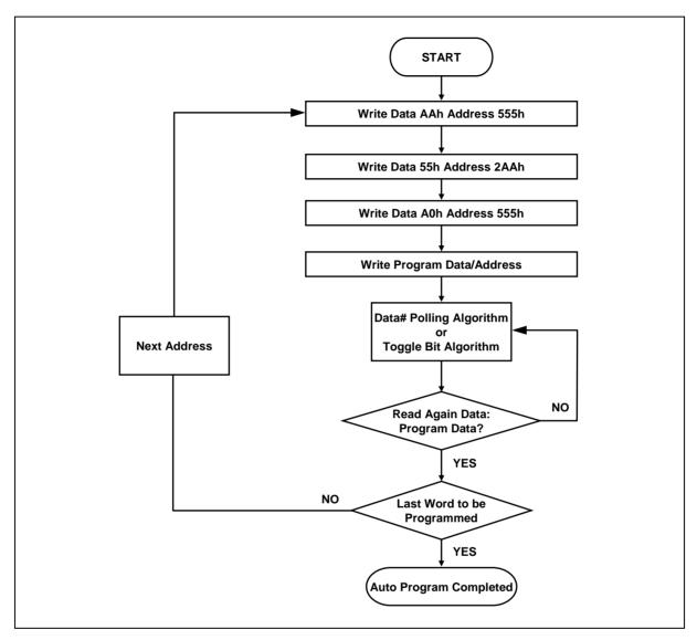
Figure 8-17 Automatic Programming Algorithm Flowchart
