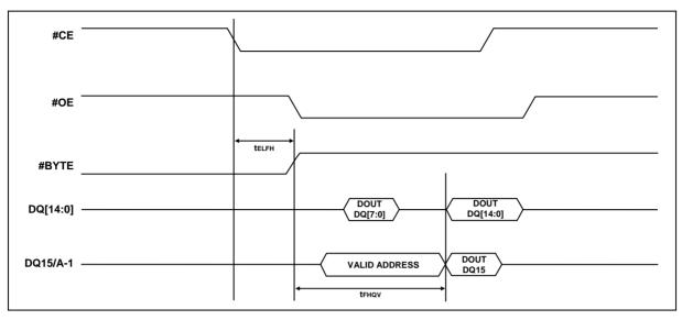
Figure 8-24 #BYTE Timing Waveform For Read operations
