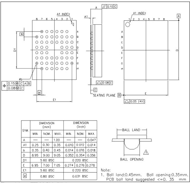
Figure 9-2 TFBGA 56-ball 7x9mm
