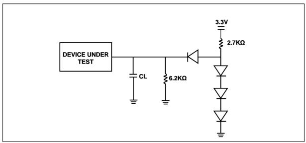
Figure 8-3 Switch Test Circuit
