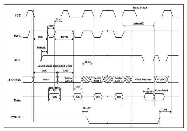
Figure 8-10 Automatic Sector Erase Timing Waveform
