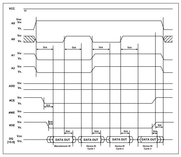
Figure 8-18 Silicon ID Read Timing Waveform
