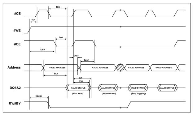
Figure 8-22 Toggling Bit Timing Waveform (During Automatic Algorithms)
