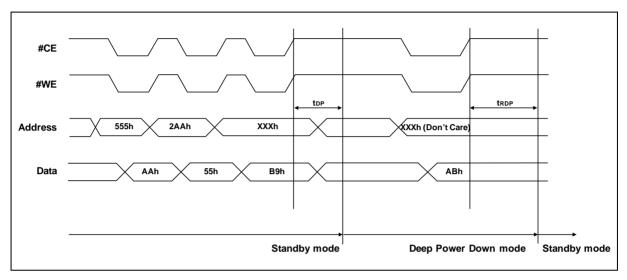
Figure 8-26 Deep Power Down mode Waveform
