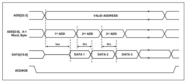
Figure 8-25 Page Read Timing Waveform
