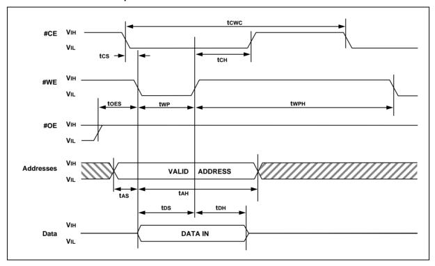
Figure 8-5 Instruction Write Operation Waveform
