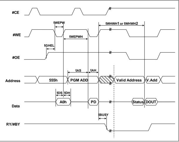
Figure 8-16 #WE Controlled Write Timing Waveform
