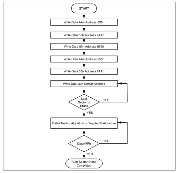
Figure 8-11 Automatic Sector Erase Algorithm Flowchart
