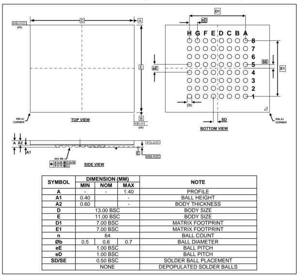
Figure 9-3 LFBGA 64-ball 11x13mm
