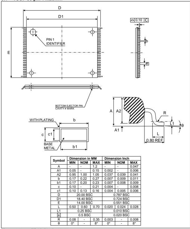
Figure 9-1 TSOP 56-pin 14x20mm
