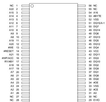
Figure 3-3 56-PIN STANDARD TSOP (TOP VIEW)
