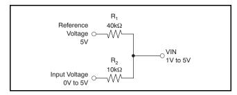
Figure 43. Resistive Divider for  $I_{MIN}$  to  $I_{MAX}$  Output (4mA to 20mA) with 0V to  $V_{FS}$  Signal Source
