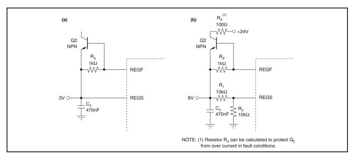
Figure 49. Voltage Regulator Current Boost Using a Standard NPN Transistor
