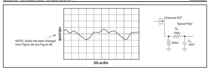
Figure 41. Output with Additional Filter
