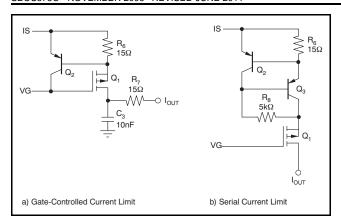
Figure 37. External Current Limit Circuits
