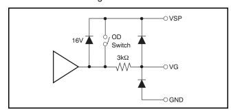
Figure 38. Equivalent Circuit for Gate Drive and Disable Switch
