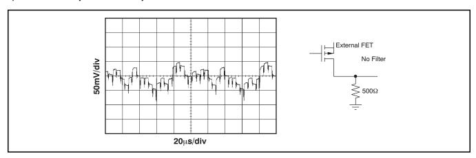
Figure 39. Output Noise without Filter into 500 $\Omega$
