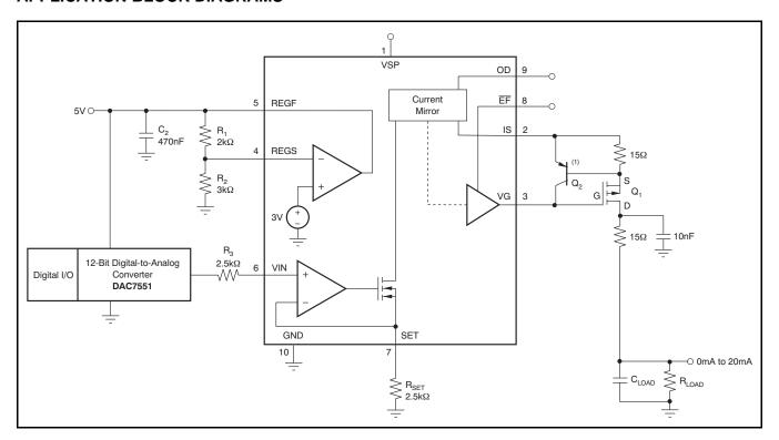
Figure 46. Current Using 0V to 5V Input from a 12-Bit Digital-to-Analog Converter DAC7551
