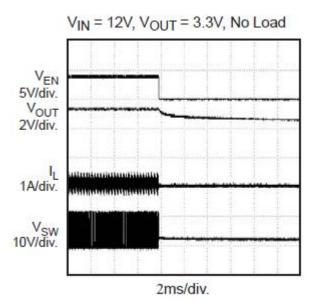
Figure 8. Shutdown through Enable
