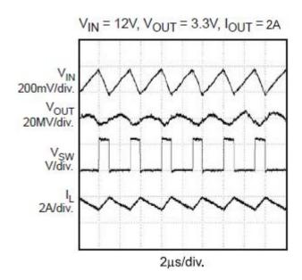
Figure 5. Steady State Test
