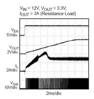
Figure 6. Startup through Enable
