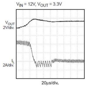
Figure 12. Short Circuit Recovery
