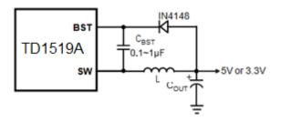
Figure 14.Add Optional External Bootstrap Diode to Enhance Efficiency
