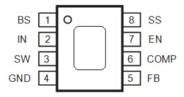
Figure 2 Pin Configuration of TD1519A(Top View)
