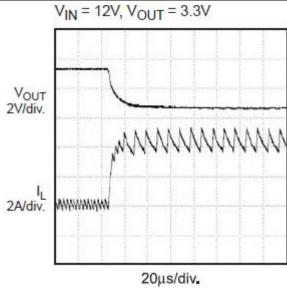
Figure 11. Short Circuit Test
