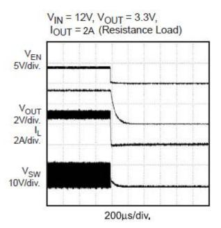
Figure 9. Shutdown through Enable
