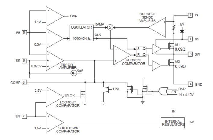
Figure 3 Function Block Diagram of TD1519A
