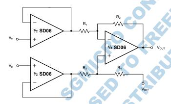
Figure 5. Instrumentation Amplifier
