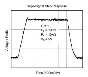
At  $T_A$  = +25°C,  $V_{CM}$  =  $V_S/2$ ,  $R_L$  = 600 $\Omega$ , unless otherwise noted.
