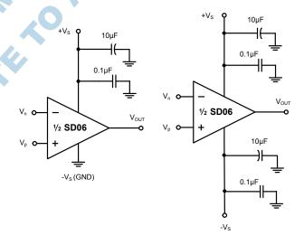
Figure 3. Amplifier with Bypass Capacitors
