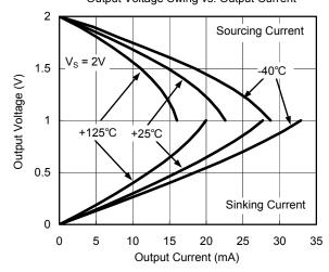
At  $T_A$  = +25°C,  $V_{CM}$  =  $V_S/2$ ,  $R_L$  = 600 $\Omega$ , unless otherwise noted.
