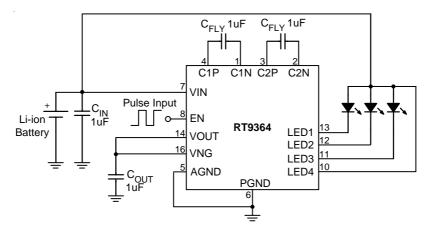
Figure 2. For 3-WLEDs Application Circuit
