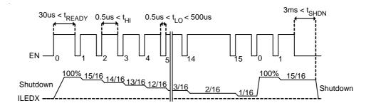
Figure 3. Brightness control by pulse dimming
