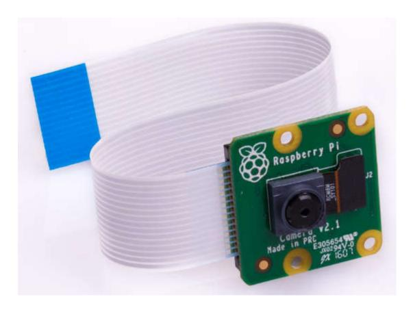
The Raspberry Pi Camera Module v2 replaced the original Camera Module in April 2016. The v2 Camera Module has a Sony IMX219 8-megapixel sensor (compared to the 5-megapixel OmniVision OV5647 sensor of the original camera).
