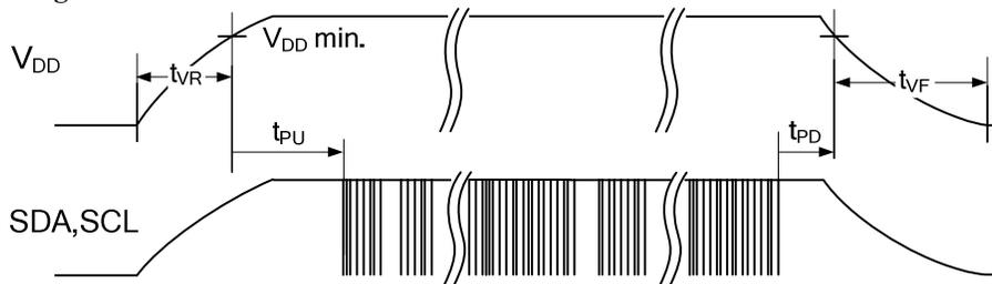
**Power Cycle Timing** ( $T_A = -40^\circ\text{C}$  to  $+85^\circ\text{C}$ ,  $V_{DD} = 4.5\text{V}$  to  $5.5\text{V}$  unless otherwise specified)
