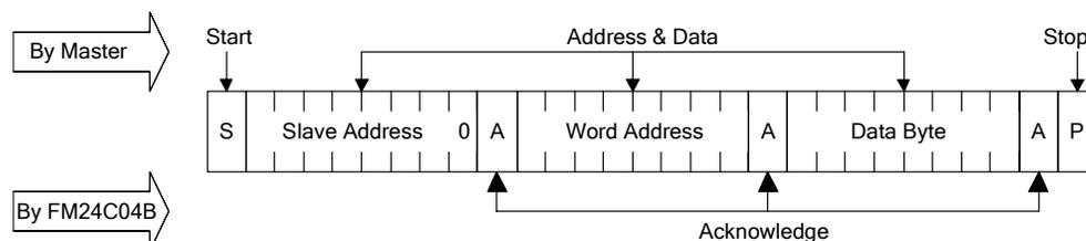
Figure 5. Byte Write
