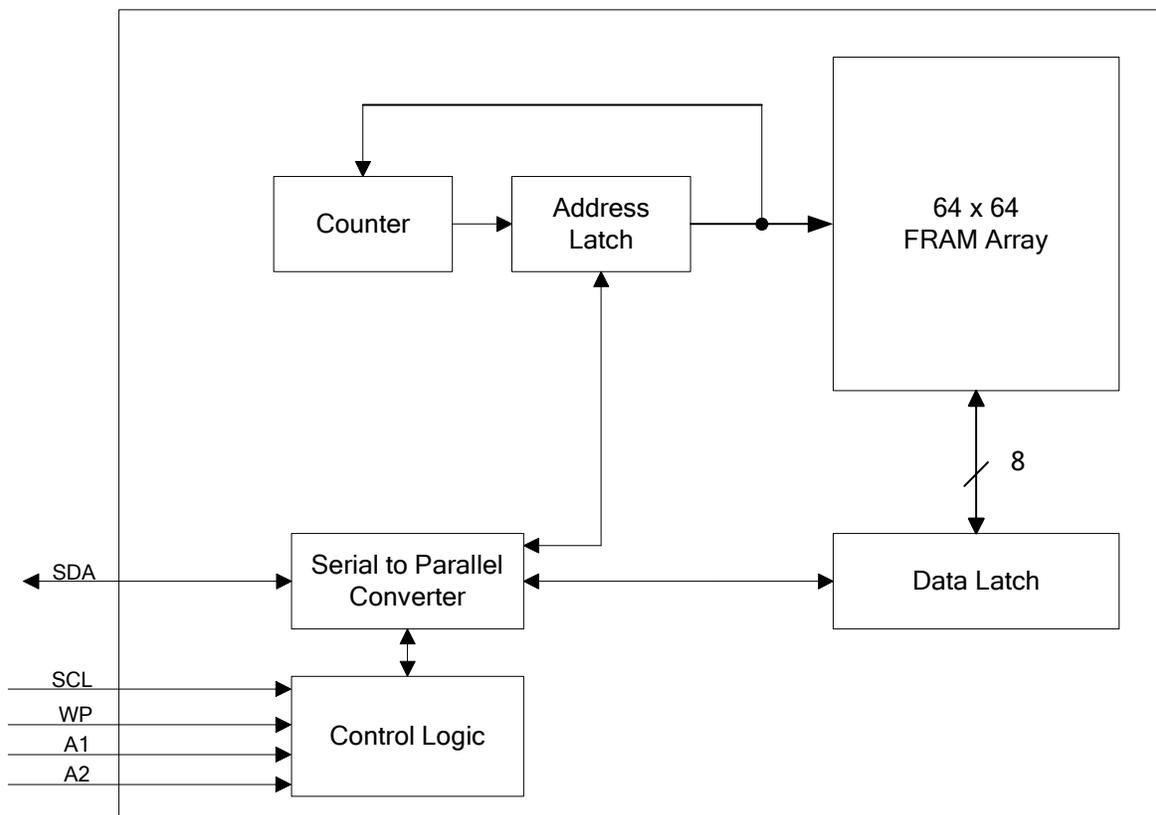
Figure 1. Block Diagram
