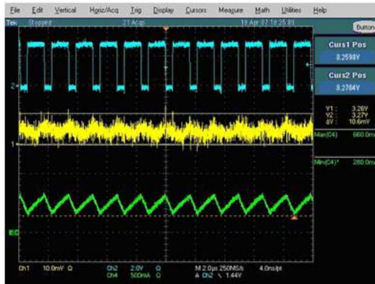
Figure 9. Ceramic 22µF 1210(X5R) (Good)
