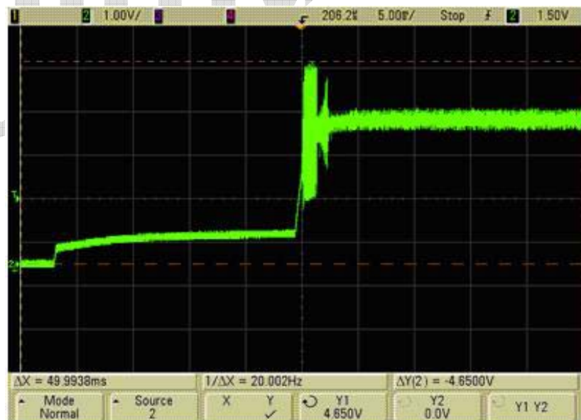
Figure 8. Input Voltage Overshoot >4V (Bad)
