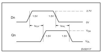
Waveform 2. Propagation Delay for Data to Outputs
