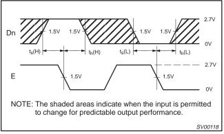
Waveform 3. Data Setup and Hold Times
