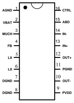
SOP16L-PP/SOP16L Top View
