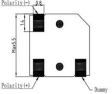
\*Unit: mm; Tolerance: ± 0.3mm Except Specified \*Housing Material: Black LCP \*Terminal plate: 3 soldering pads, tin Plating Brass
