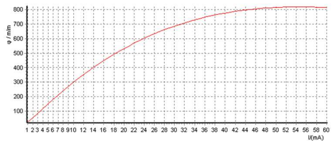
电流-光通量曲线 Current-Luminous flux Curve
