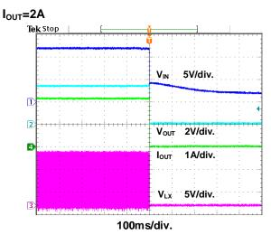
Figure 10. Power Off through VIN Waveform
