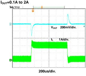
Figure 15. Load Transient Waveform
