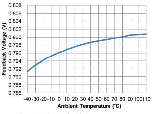
Figure 20. Feedback Voltage vs. Temperature
