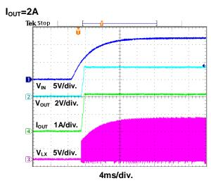
Figure 8. Power On through VIN Waveform
