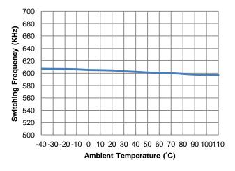
Figure 21. Switching Frequency vs. Temperature
