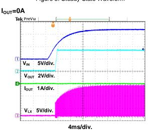
Figure 7. Power On through VIN Waveform
