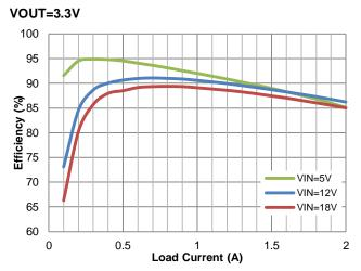
Figure 18. Efficiency vs. Load Current
