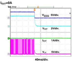
Figure 13. Power Off through SHDN Waveform
