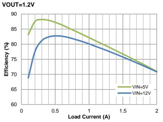
Figure 17. Efficiency vs. Load Current
