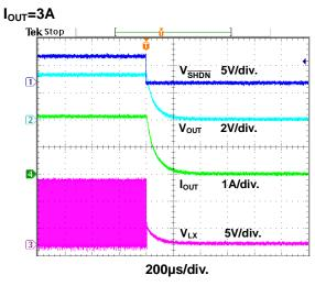
Figure 14. Power Off through SHDN Waveform
