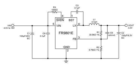
Figure 3. C<sub>IN</sub>/C<sub>OUT</sub> use Electrolytic Capacitors Application Circuit
