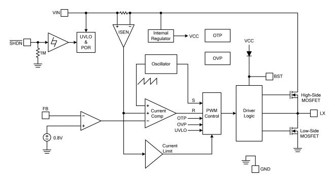
Figure 4. Block Diagram of FR9801E
