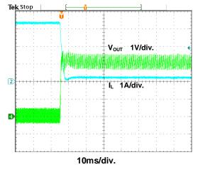
Figure 16. Short Circuit Test
