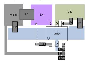
Figure 22. Recommended Layout Diagram
