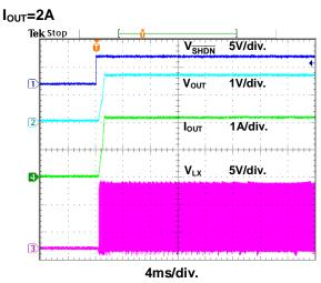
Figure 12. Power On through SHDN Waveform
