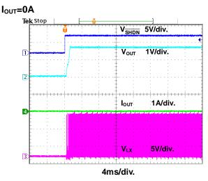
Figure 11. Power On through SHDN Waveform
