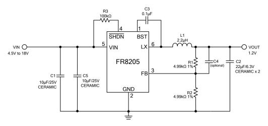
Figure 2. C<sub>IN</sub>/C<sub>OUT</sub> use Ceramic Capacitors Application Circuit
