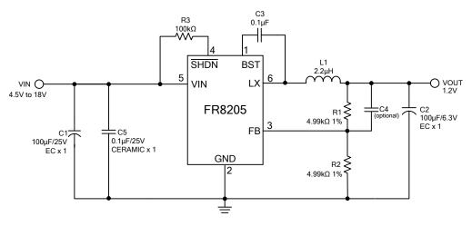
Figure 3.  $C_{\text{IN}}/C_{\text{OUT}}$  use Electrolytic Capacitors Application Circuit
