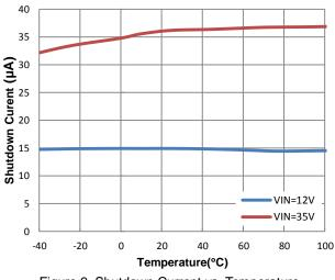
Figure 9. Shutdown Current vs. Temperature
