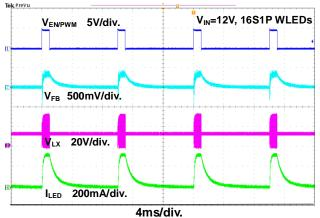
Figure 13. PWM Dimming Response Waveforms at a frequency of 100Hz(Duty10%)
