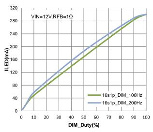
Figure 6. LED Current vs. Duty Cycle(B Version)
