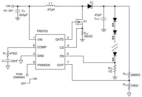
Figure 2. Typical Application Circuit of FP6753A without exposed pad
