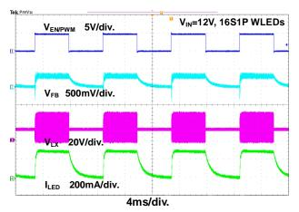
Figure 14. PWM Dimming Response Waveforms at a frequency of 100Hz(Duty50%)
