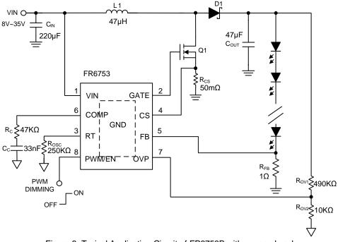
Figure 3. Typical Application Circuit of FP6753B with exposed pad
