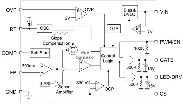
Figure 5. Block Diagram of FP6753
