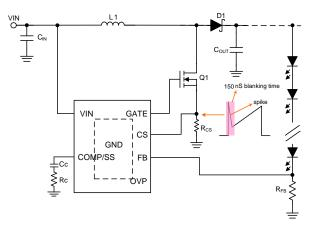
Figure17. With blanking time
