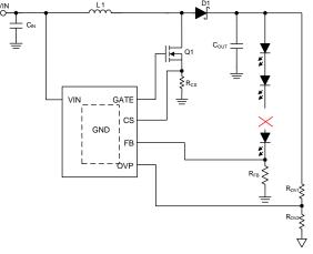
Figure 16. With Open-Circuit Protection
