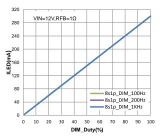
Figure 7. LED Current vs. Duty Cycle(C Version)
