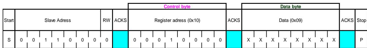
Figure 26: I<sup>2</sup>C write
