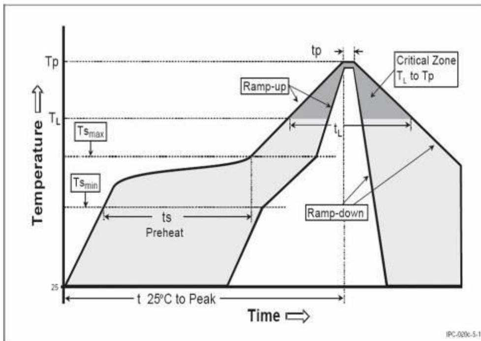
Figure 37: Soldering profile
