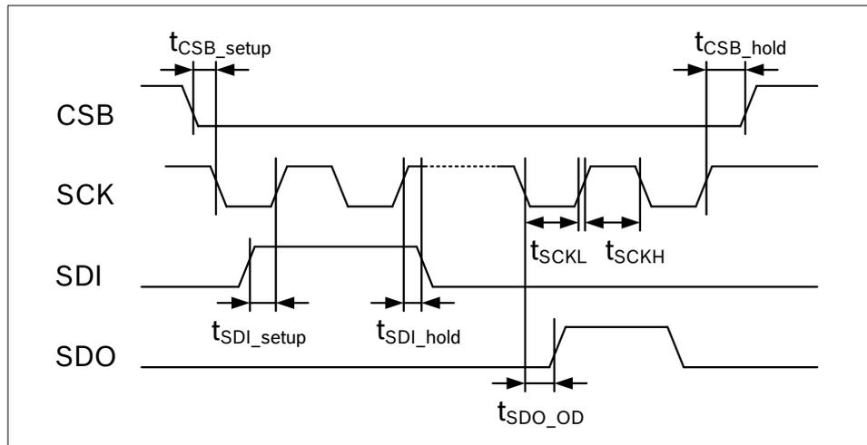
Figure 20: SPI timing diagram
