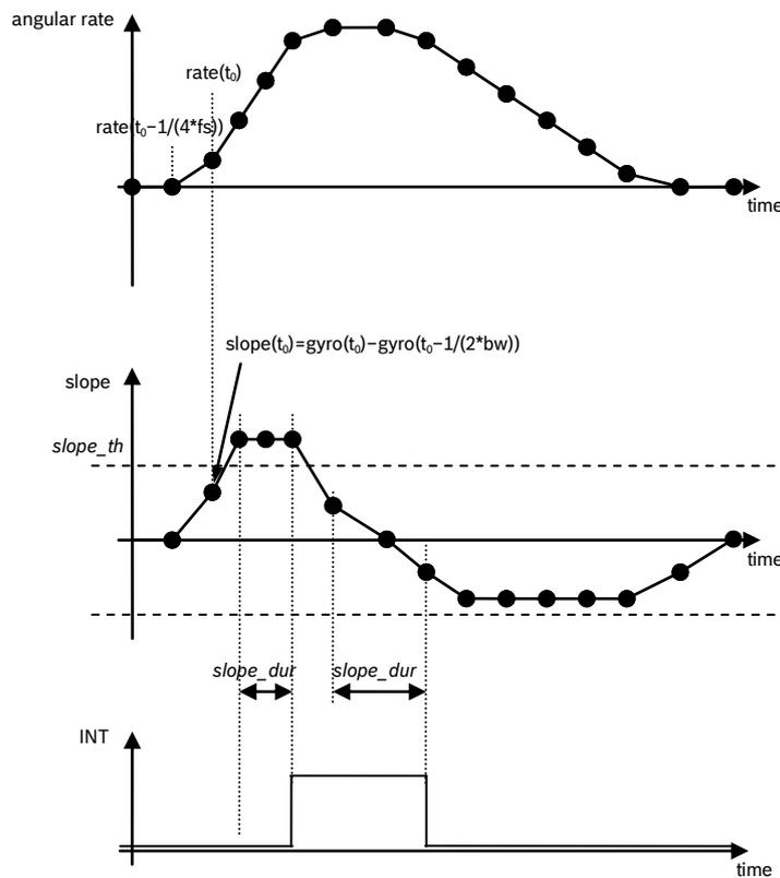
Figure 17: Principle of any-motion detection,(will be updated)
