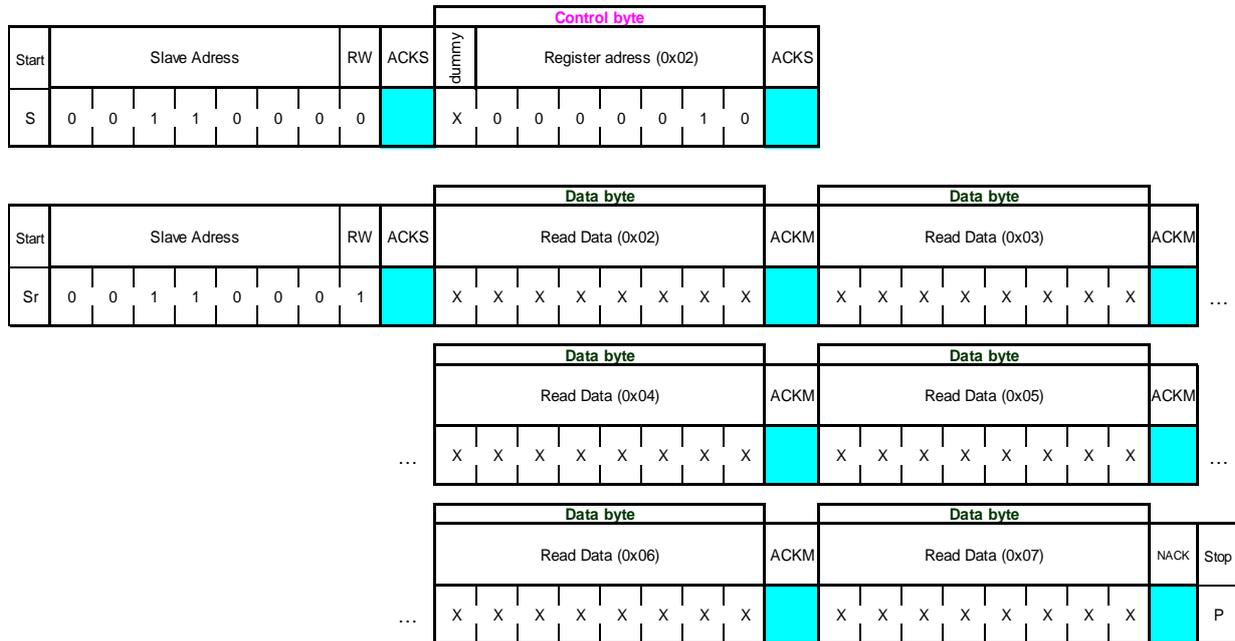
Figure 27: I<sup>2</sup>C multiple read
