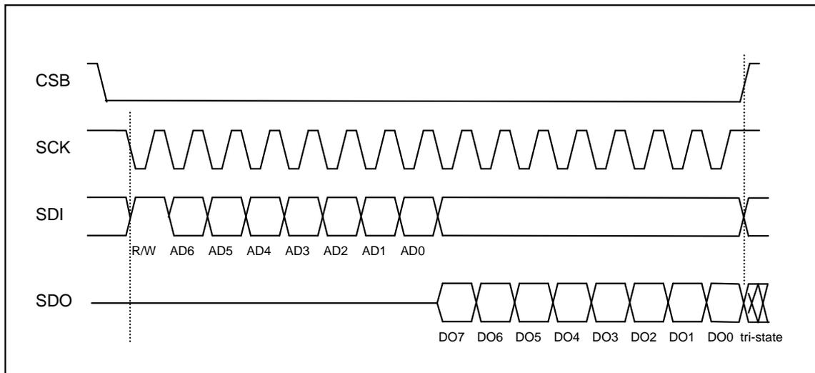
Figure 22: 4-wire basic SPI read sequence (mode '11')
