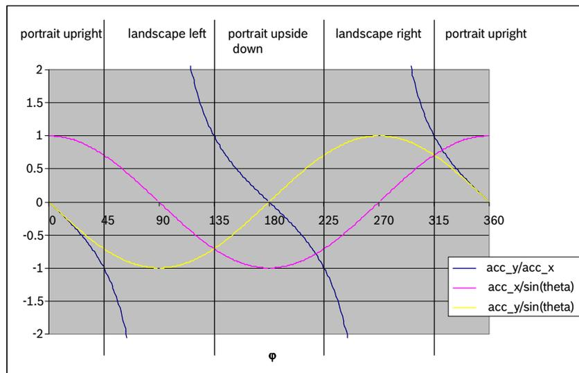
Figure 10: Typical orientation switching conditions w/o hysteresis
