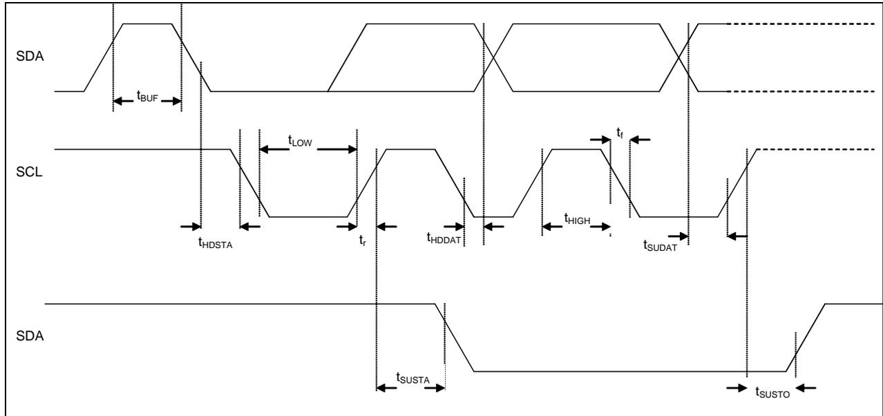
Figure 25: I<sup>2</sup>C timing diagram
