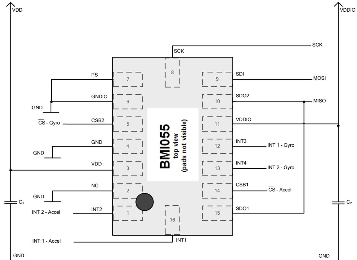
Figure 31: 4-wire SPI connection
