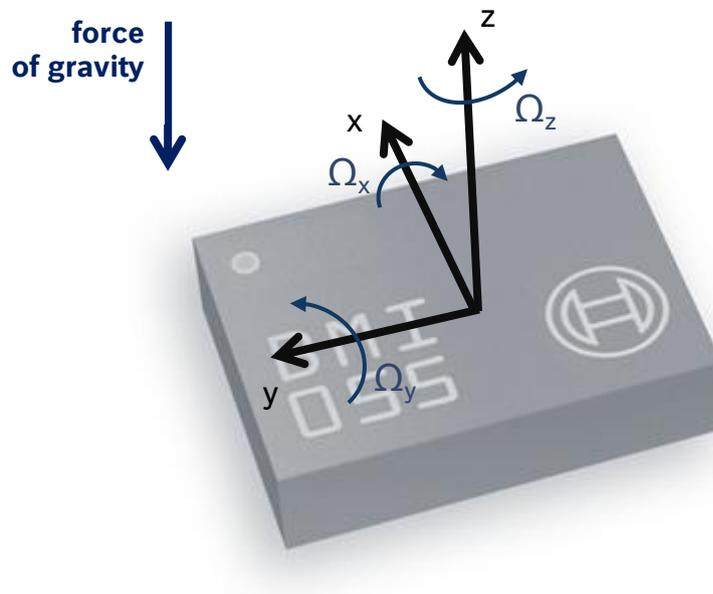
Figure 35: Orientation of sensing axis
