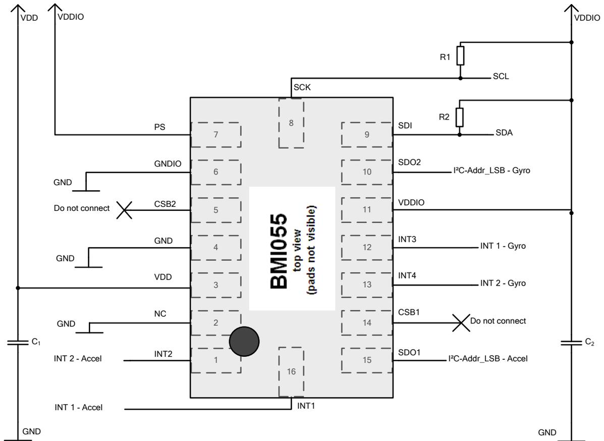
Figure 33: I<sup>2</sup>C connection
