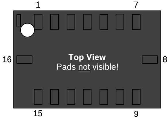
Figure 29: Pin-out top view
