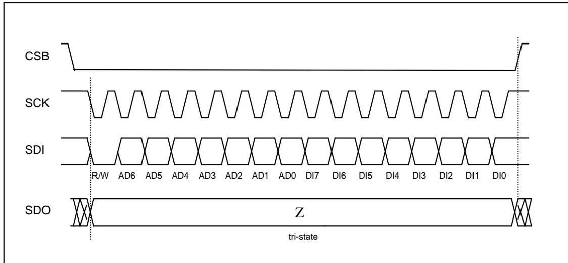
Figure 21: 4-wire basic SPI write sequence (mode '11')
