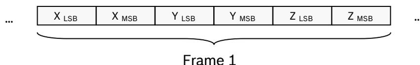
If only one axis is enabled, the format of the data read-out from (*ACC 0x3F*) is as follows (example shown: y-axis only, other axes are equivalent).
