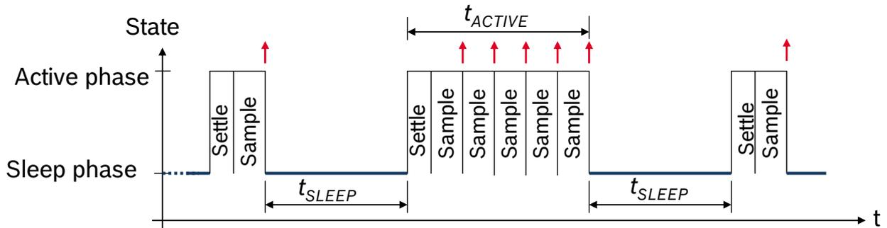
Figure 3: Timing Diagram for low-power mode 1/2, EDT
