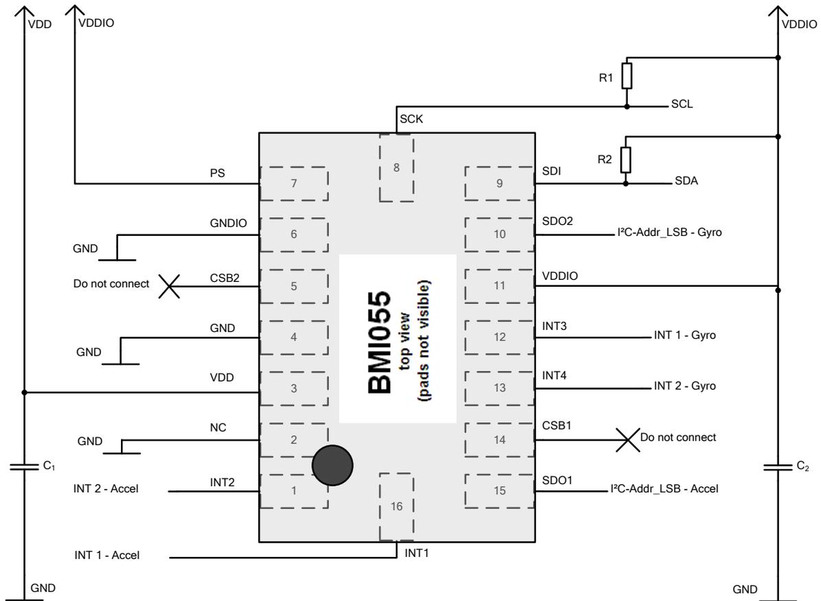
Figure 33: I<sup>2</sup>C connection
