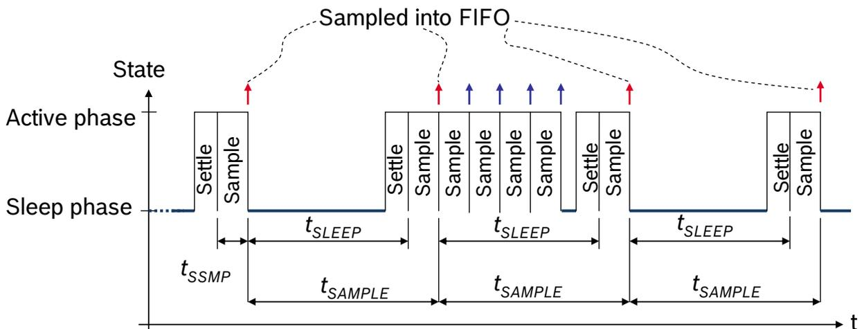
Figure 4: Timing Diagram for low-power mode 1/2, EST
