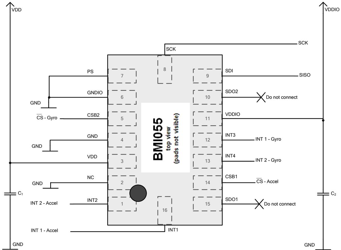
Figure 32: 3-wire SPI connection
