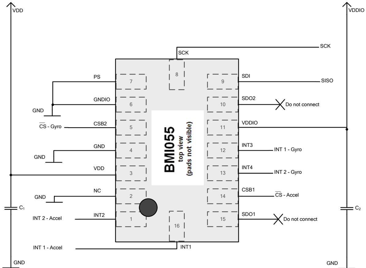
Figure 32: 3-wire SPI connection
