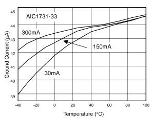
Fig. 5 Ground Current vs. Temperature
