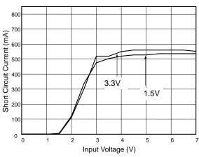
Fig. 4 Input Voltage vs. Short Circuit Current
