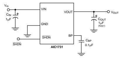
**Low Noise Low Dropout Linear Regulator**
