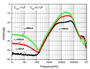
Fig. 18 Ripple Rejection
