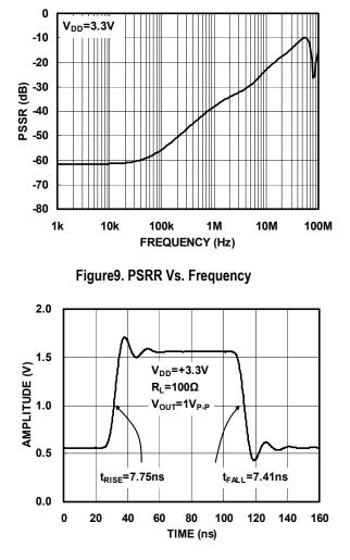
Figure11. Large-Signal Pulse Response Vs. Time
