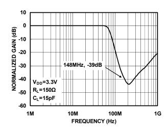
Figure8. Stop Band Attenuation
