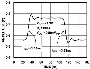
Figure12. Small-Signal Pulse Response Vs. Time
