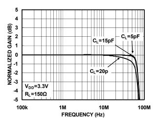
Figure5. Gain Vs. Frequency With CLOAD
