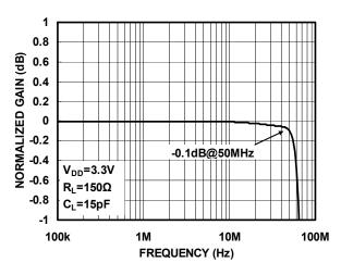
Figure3. Small-Scale Frequency Response
