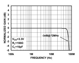
Figure4. Large-Scale Frequency Response
