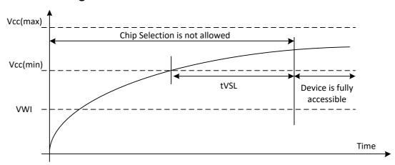
**Power-Up Timing and Write Inhibit Threshold**
