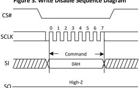
Figure 3. Write Disable Sequence Diagram
