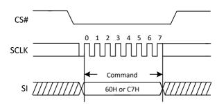
Figure 13. Chip Erase Sequence Diagram
