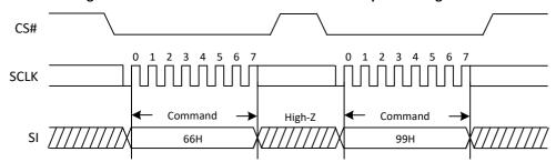
Figure 22. Enable Reset and Reset command Sequence Diagram
