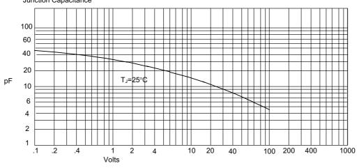
Junction Capacitance - pF*versus* Reverse Voltage - Volts
