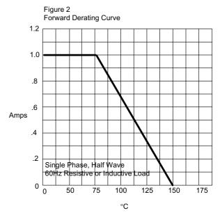
Average Forward Rectified Current - Amperes/ersus Ambient Temperature - $^{\circ}$ C
