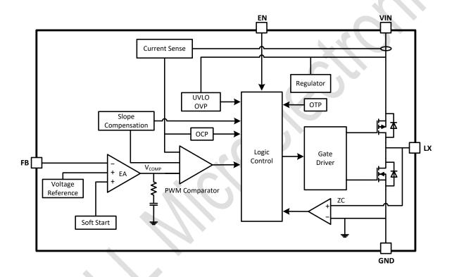
Figure 2. TM108JD Block Diagram
