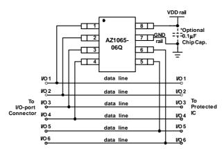
Fig. 2 Data lines and power rails connection of AZ1065-06Q.
