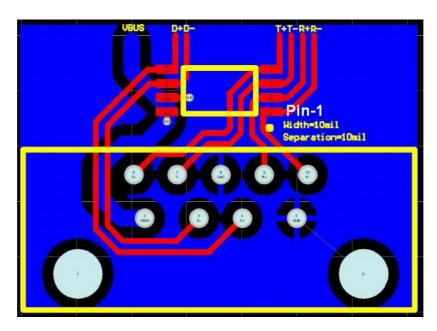
Fig. 4 USB3.0 ESD Protection by using AZ1065-06Q.
