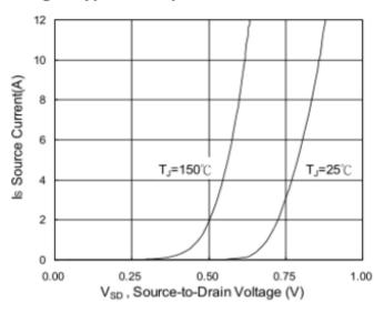
Fig.3 Forward Characteristics of Reverse Diode
