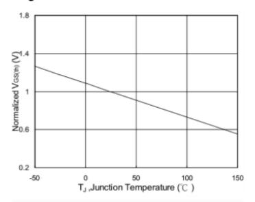
Fig.5 Normalized V<sub>GS(th)</sub> vs. T<sub>J</sub>
