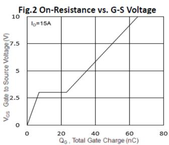
Fig.4 Gate-Charge Characteristics
