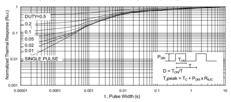
Fig.9 Normalized Maximum Transient Thermal Impedance
