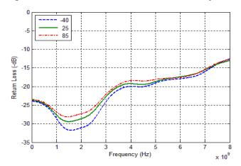
Figure 9. RFC Port Return Loss vs. V<sub>DD</sub>
