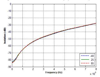
Figure 17. Isolation vs. V<sub>DD</sub> (RFC-RFX)
