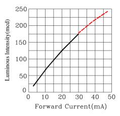
Fig.3 Luminous Intensity vs.Forward Current
