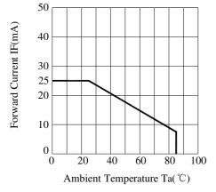
Fig.6 Forward Current Derating Curve
