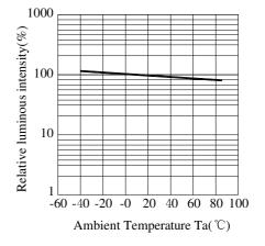
Fig.5 Luminous Intensity vs.Ambient Temperatur
