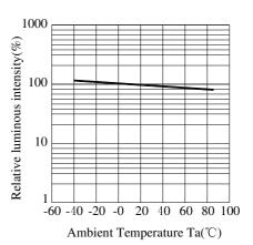
Fig.5 Luminous Intensity vs.Ambient Temperature
