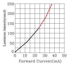
Fig.3 Luminous Intensity vs.Forward Current
