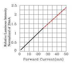
Fig.4 Relative Luminous Intensity vs.Forward Current
