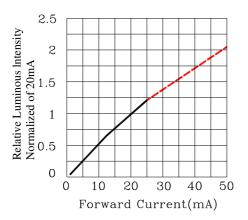
Fig.4 Relative Luminous Intensity vs.Forward Current
