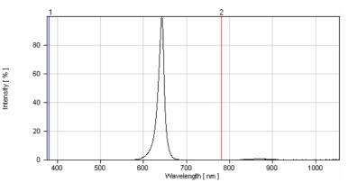
Fig.1 Red Relative Intensity vs. Wavelength
