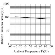
Fig.5 Luminous Intensity vs.Ambient Temperature
