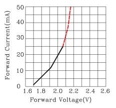
Fig.2 Forward Current vs.Forward Voltage
