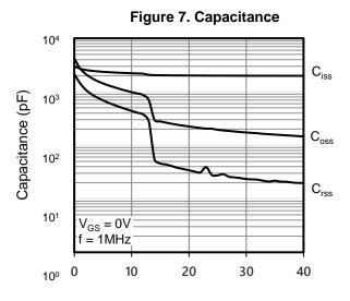
$V_{DS}$ , Drain-to-Source Voltage (V)
