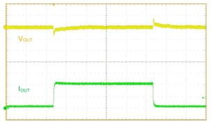
$V_{IN}$  = 12V,  $V_{OUT}$  = 0.9V, 100 $\mu$ s/div  $V_{OUT}$ : 30mV/div,  $I_{OUT}$ : 10A/div, 10A/ $\mu$ s
