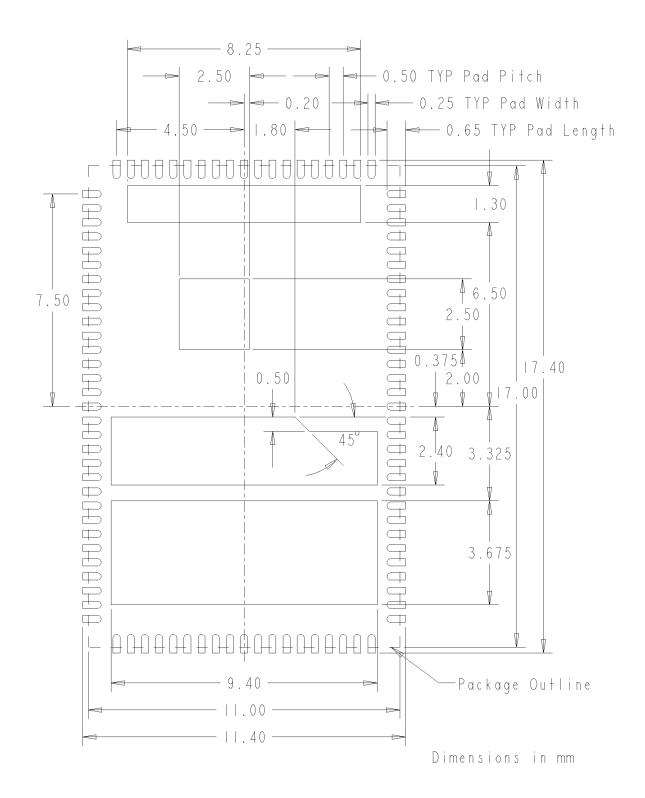
**Figure 20: Recommended PCB Footprint**
