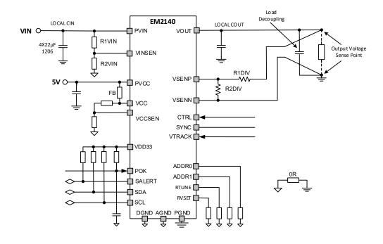
**Figure 15: Recommended Application Circuit**
