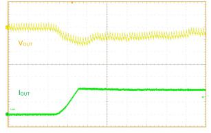
$V_{IN}$  = 12V,  $V_{OUT}$  = 0.9V, 10 $\mu$ s/div  $V_{OUT}$ : 10 mV/div,  $I_{OUT}$ : 10A/div, 1A/ $\mu$ s
