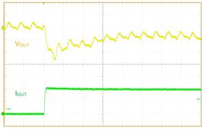
$V_{IN}$  = 12V,  $V_{OUT}$  = 0.9V, 2 $\mu$ s/div  $V_{OUT}$ : 10mV/div,  $I_{OUT}$ : 10A/div, 10A/ $\mu$ s
