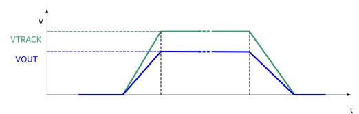
Figure 13: Ratiometric Sequencing Using VTRACK
