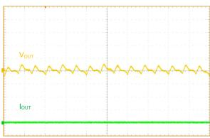
$V_{IN}$  = 12V,  $V_{OUT}$  = 0.9V 2  $\mu$ s/div,  $V_{OUT}$ : 10 mV/div, 20 MHz bandwidth
