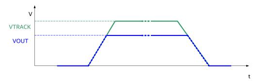
**Figure 13: Simultaneous Sequencing Using VTRACK**
