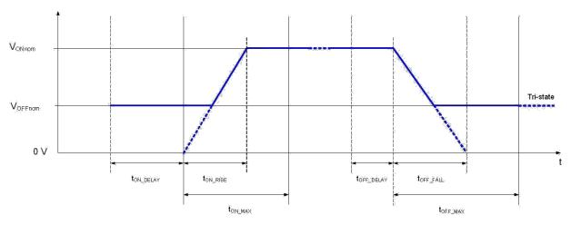
Figure 8: Power Sequencing With Non-Zero Off Voltage
