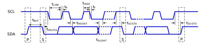
Figure 14: PMBus Timing Diagram
