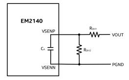
**Figure 5: Output Voltage Sense Circuitry**
