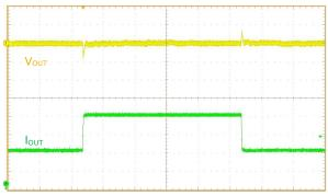
$V_{IN}$  = 12V,  $V_{OUT}$  = 0.9V, 100 $\mu$ s/div  $V_{OUT}$ : 30mV/div,  $I_{OUT}$ : 10A/div, 10A/ $\mu$ s
