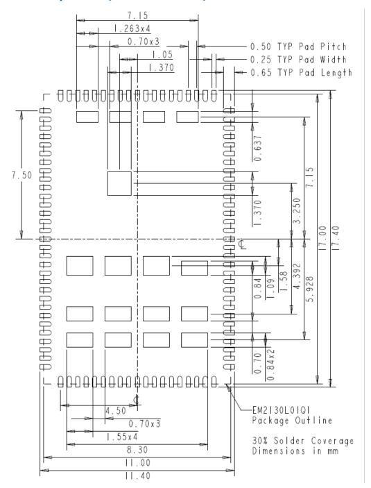
Figure 21: 30% Solder Stencil Aperture Dimensions
