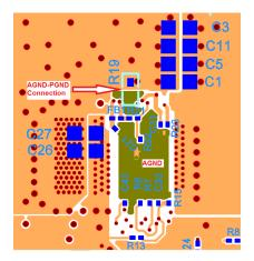
Figure 18: Backside Decoupling
