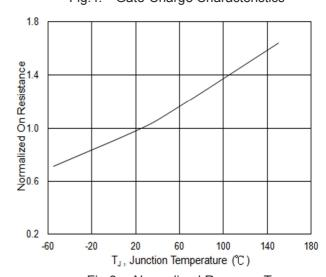
Fig.6: Normalized R<sub>DSON</sub> vs. T<sub>J</sub>
