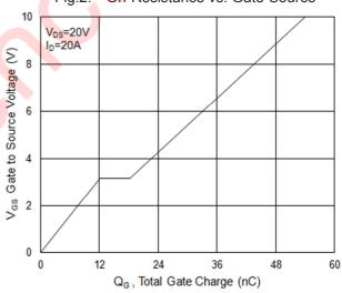
Fig.4: Gate-Charge Characteristics
