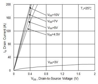
Fig.1: Typical Output Characteristics
