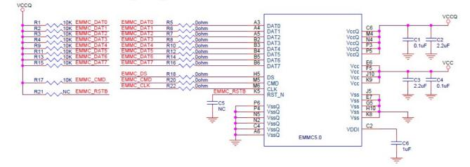
The resistance on the CLK line is highly recommended (0 $\Omega$  by default)
