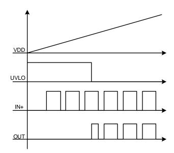
Figure 11. SCT52241 Non-inverting Output Vs VDD
