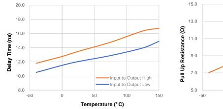
Figure 7. Input to Output Propagation Delay vs Temperature
