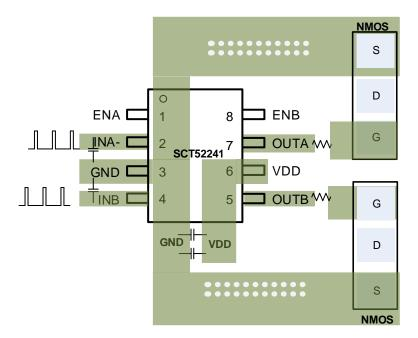
Figure 19. SCT52241 PCB Layout Example
