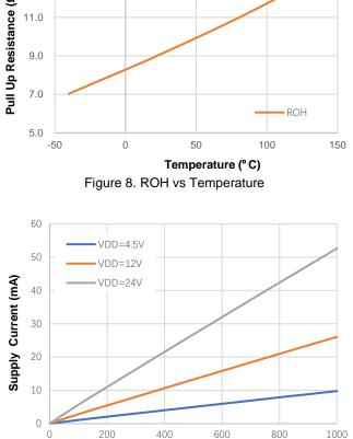
Figure 10. Operation Supply Current vs Frequency, Cout=1nF
