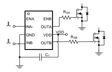
Figure 16. Dual Channel Driver Typical Application
