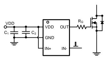
Figure 20. SCT51240 Inverting MOSFET Gate Drive Typical Application
