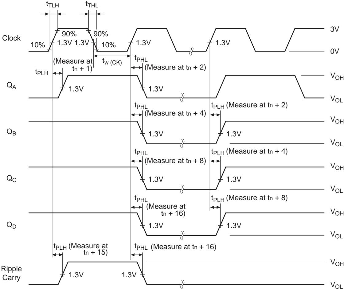
Note: Clock input pulse;  $t_{TLH} \leq 15$  ns,  $t_{THL} \leq 6$  ns, PRR = 1 MHz, duty cycle 50% and :  $f_{max} t_{TLH} = t_{THL} \leq 2.5$  ns.
