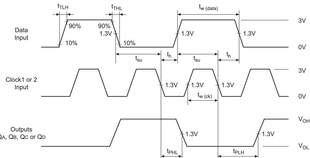
Note: Input pulse;  $t_{TLH}, t_{THL} \leq 10$  ns, Data PRR = 500 kHz, Clock PRR = 1 MHz,
