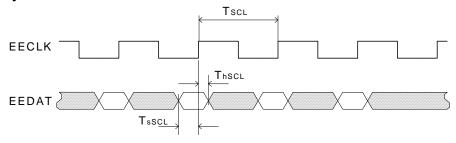
Command cycle EEPROM Timing Tx Parameters
