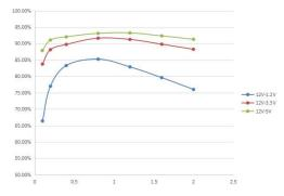
2.Efficiency(%) vs. Load Current(A)
