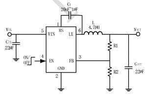
Figure 1. Basic Application Circuit
