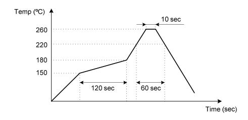
Note: Total Time: 200 sec. Max., Solder Melting Point: 220°C
