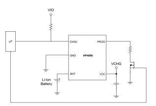
The HP4056 also be put into shutdown mode when VCC voltage down to UVLO threshold. In this state, the CHGb pin is high impedance state. The CHGb pin is also in a high impedance state if the charge cycle is completed.
