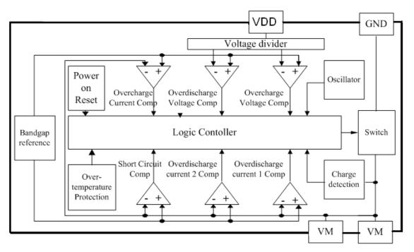
Figure 3. Functional Block Diagram
