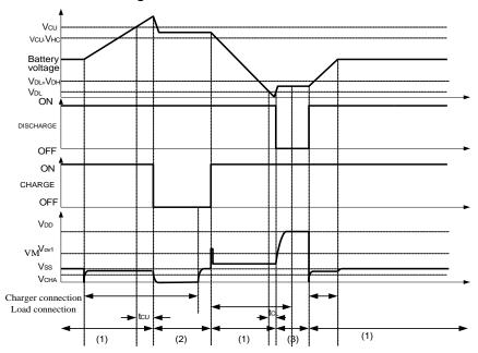
Figure 5-1 Overcharge and Overdischarge Voltage Detection
