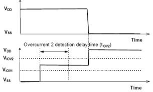
Figure 4. Overcurrent delay time
