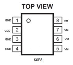
Figure 2. PIN Configuration
