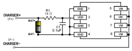
Fig 6 XB8608A2 in a Typical Battery Protection Circuit
