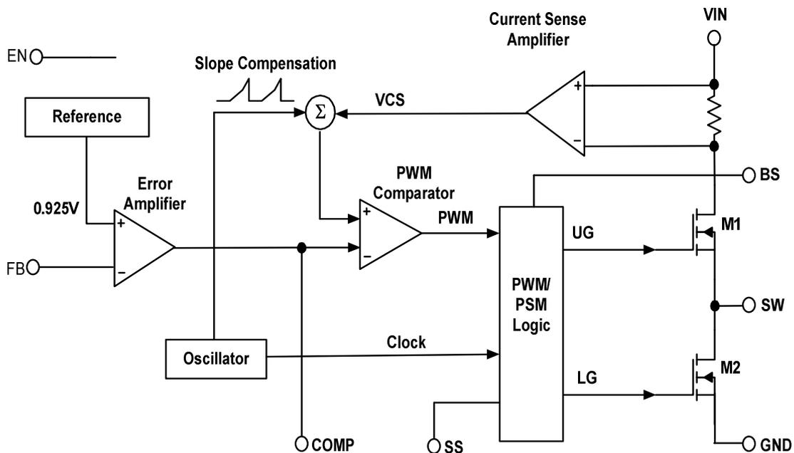
**Figure 2. IT76620M Functional Block Diagram**
