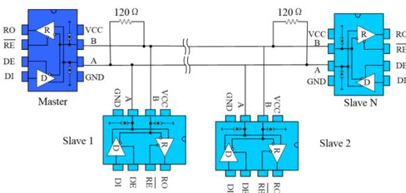
Backbone cable type RS485 communications network
