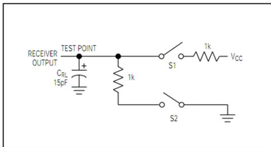
Fig 8 Receiver Enable/Disable Timing Test Load
