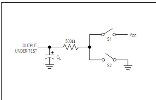
Fig 4 Driver Enable/Disable Timing Test Load
