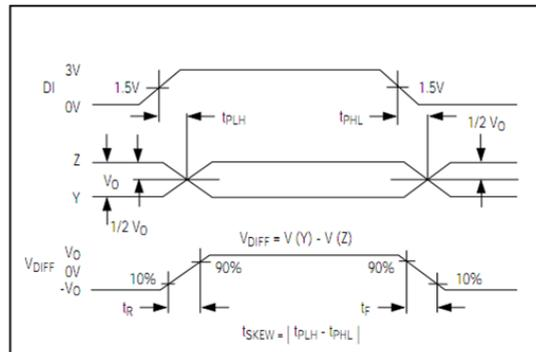
Fig 3 Driver Propagation Delays
