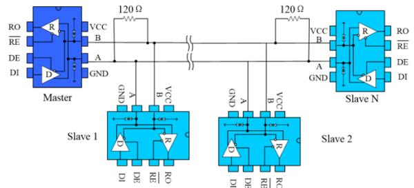
Fig 10 Backbone cable type RS485 communications network
