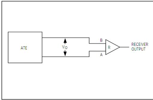
Fig 6 Receiver Propagation Delay Test Circuit
