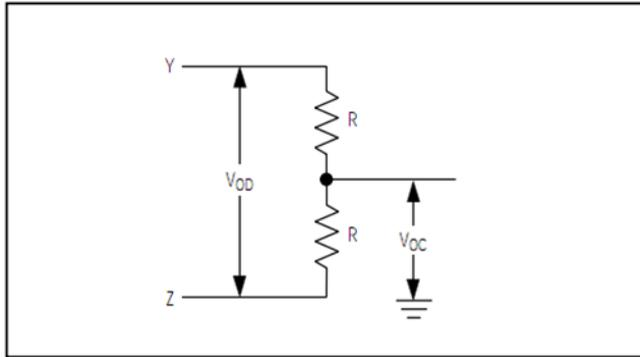
Fig 1 Driver DC Test Load
