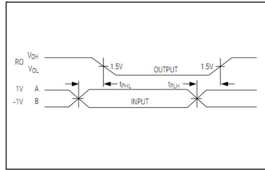
Fig 7 Receiver Propagation Delays
