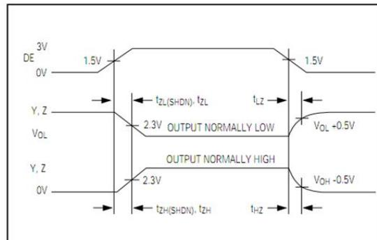
Fig 5 Driver Enable and Disable Times
