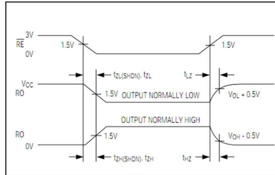
Fig 9 Receiver Enable and Disable Times
