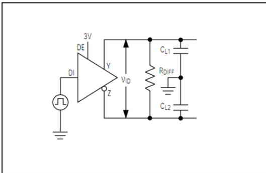
Fig 2 Driver Timing Test Circuit
