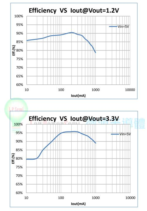
$(V_{IN}=V_{EN}=5V,L=2.2uH,C_{IN}=10uF,C_{OUT}=10uF,T_{A}=25^{\circ}C$ , unless otherwise noted)
