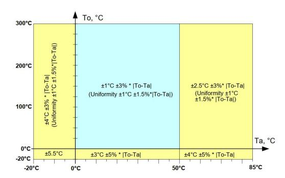
Figure 4 Temperature measurement accuracy for normal objects
