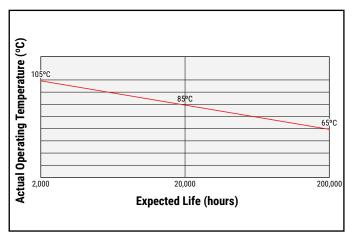
The effect of derating temperature can be seen in this graph.
