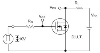
Fig. 2.1 Switching Test Circuit
