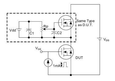
Fig. 3 . 1 Gate Charge Test Circuit
