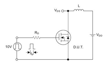
Fig. 4.1 Unclamped Inductive Switching Test Circuit
