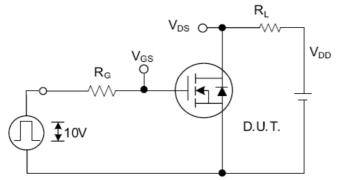
Fig. 2.1 Switching Test Circuit
