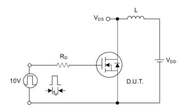
Fig. 4.1 Unclamped Inductive Switching Test Circuit
