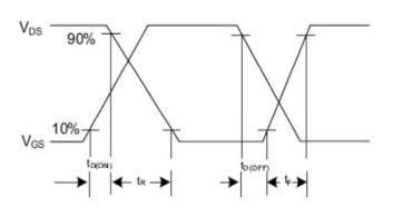
Fig. 2.2 Switching Waveforms
