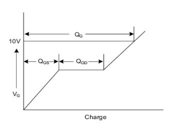
Fig. 3.2 Gate Charge Waveform
