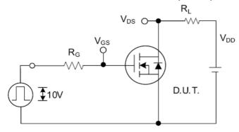
Fig. 2.1 Switching Test Circuit
