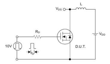
Fig. 4.1 Unclamped Inductive Switching Test Circuit
