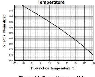
Figure 12. Threshold Voltage vs
