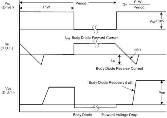
Fig. 1.2 Peak Diode Recovery dv/dt Waveforms
