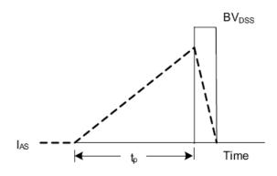
Fig. 4.2 Unclamped Inductive Switching Waveforms
