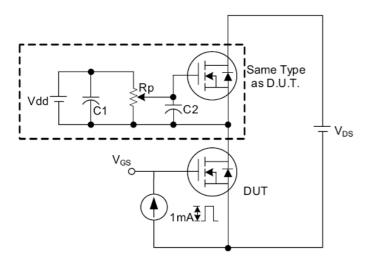
Fig. 3 . 1 Gate Charge Test Circuit
