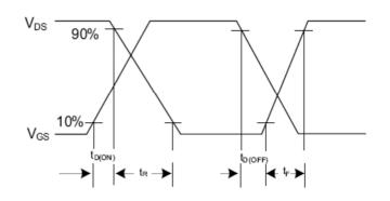
Fig. 2.2 Switching Waveforms
