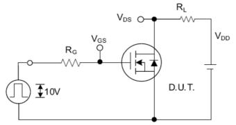
Fig. 2.1 Switching Test Circuit
