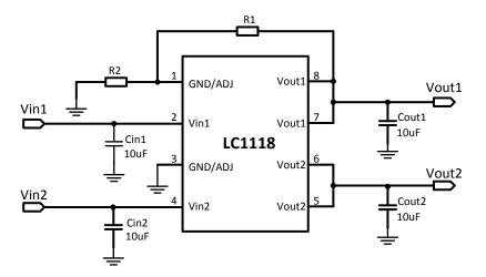
Fig.3. Typical application schematic of LC1118
