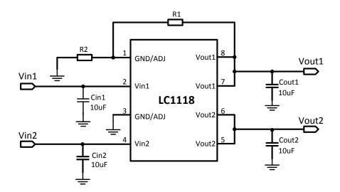
Fig.1. Typical application of LC1118
