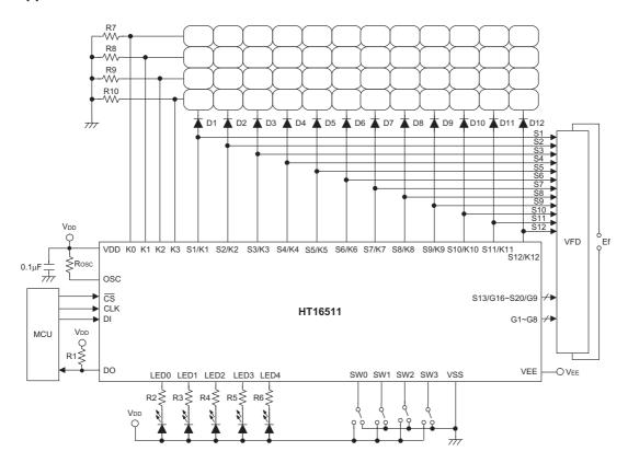
Note:  $R_{OSC}$ =51k $\Omega$  for oscillator resistor
