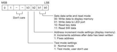
Note: power-on status: normal mode operation and address increment mode are set.
