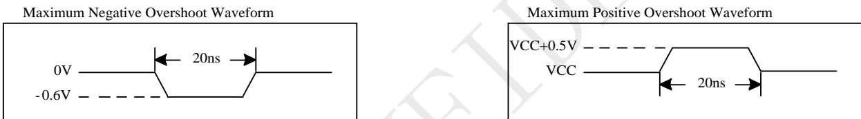
Figure 5-1 Maximum Overshoot Waveform
